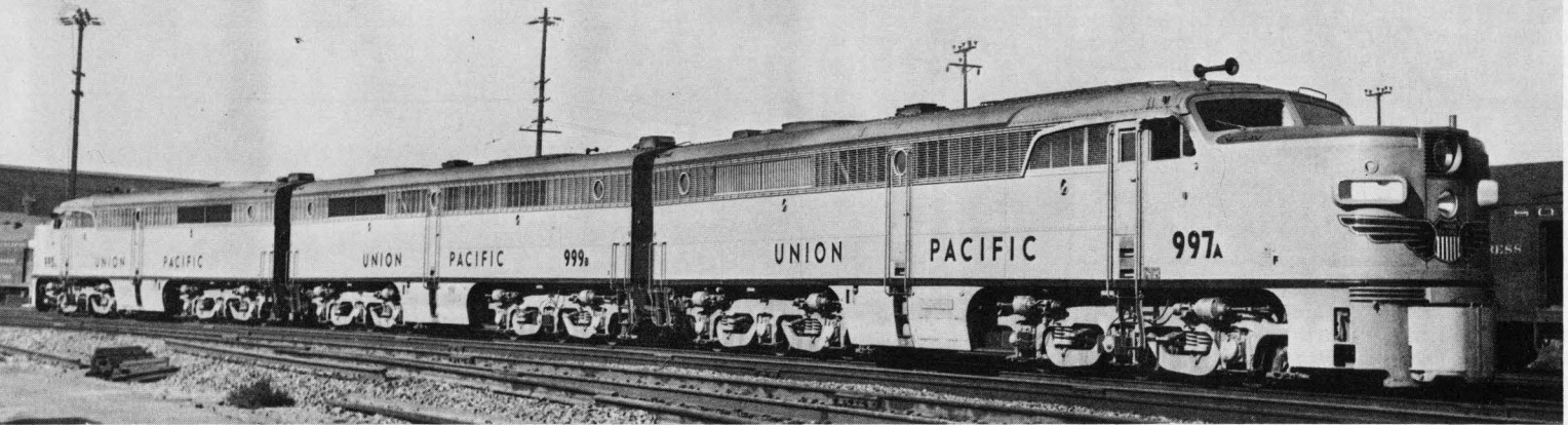
An absolutely gorgeous shot of brand new PA/B/A1 set #997A/999B/995A in Los Angeles, CA, 10/47, possibly having just completed its maiden trip. Note the coupler shroud common on most passenger diesels until the early 1950's. All of UP's went into freight service in 1955 after regearing.
