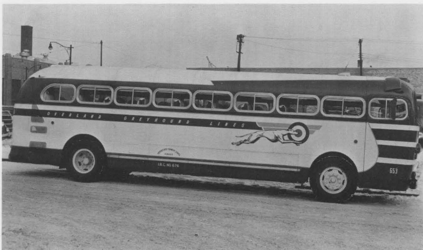
Aerocoach resumed production of its Mastercraft bus in April 1944 after a short wartime hiatus and constructed more than 1500 buses to this design between then and 1947, all with the company's trademark tubular aluminum frame, the early ones with steel body panels, later ones aluminum. Most intercity carriers had at least a few.
