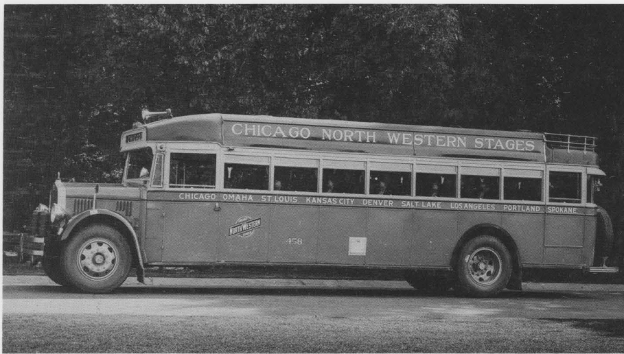
Along with Yellows and ACF's, Interstate Transit Lines took delivery of 10 additional Whites in May 1930, these of the new 54-A type, and here is one of them lettered Chicago North Western Stages for use east of Omaha. —Greyhound collection
