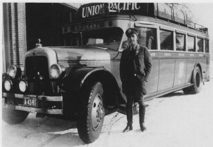
With the 1929 purchase of the Interstate Coach Co. of Spokane, Union Pacific Stages acquired a fleet of Yellow Coach type Y's; this one was photographed at Spokane in 1931. The enclosed roof bins were added locally.
