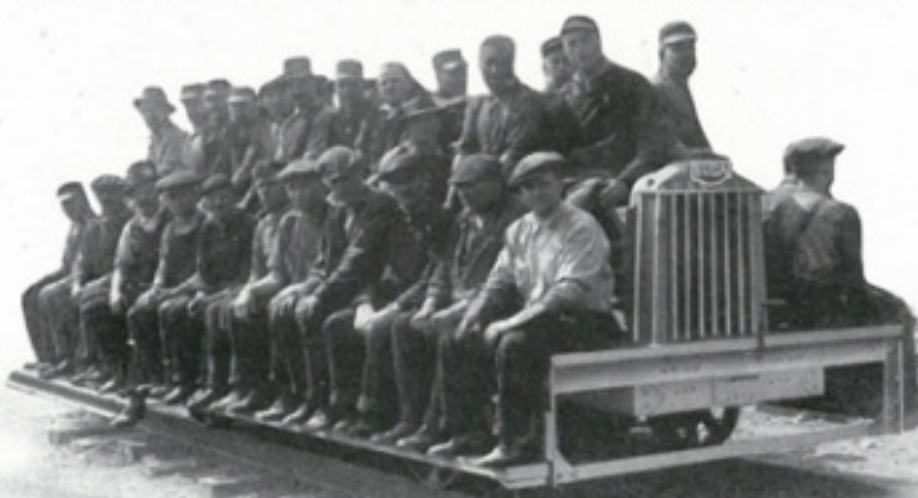
16-Passenger Inspection Car—Body Built on Buda Chassis by Railroad
