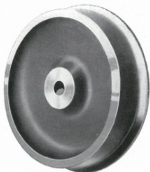
Solid Forged Steel Wheel—M. C. B. Tread and Flange
