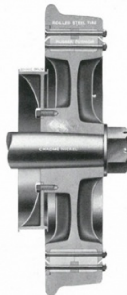
Cross Section of Rubber Cushioned Wheel—M. C. B. Tread and Flange
